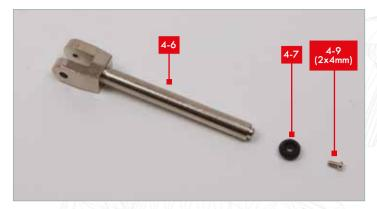
Next repeat the process with arm rod part 4-6, rubber washer 4-7 and a PM 2x4mm screw (4-9). Again note that the recess on one side of the washer fits over the end of the rod 4-6.
