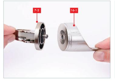
**STEP 3** Fit lower arm A **16-1** on to the peg at the centre of the arm joint.
