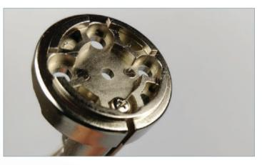
**STEP 12** The screw should sit below the rim of the area around it, as shown.
