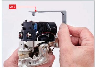
STEP 7 Align the bracket **20-3** with the top of the head.
