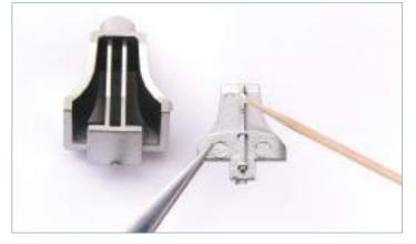
**STEP 2** Apply a little superglue to the raised spine on the smaller part.
