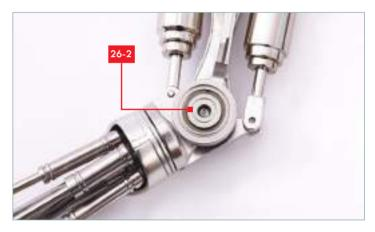
**STEP 16** Fix part **26-2** into the center of the elbow joint as shown.
