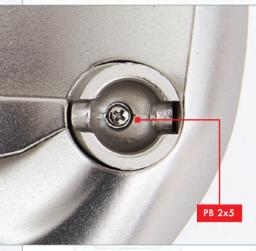
**STEP 4** Fix each of the sockets in place with a **PB** 2 x 5mm screw.
