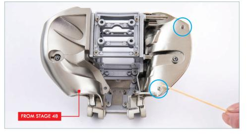
Take the assembly from stage 48. Identify the two pegs on the left side of the pelvis (circled), and after test-fitting, apply a little superglue around the sides. Fit the left pelvic shield **49-1** in place, as described in the previous stage for the right shield.
