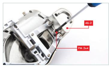
**STEP 7** Fix part **46-2** in place with a **PM** 2 x 4mm screw.
