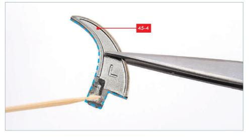
Apply a very small amount of superglue to the edges of part **45-4** that will be in contact with the assembly (highlighted with a blue dotted line).
