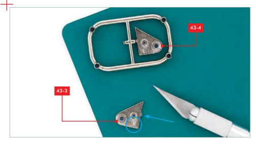
Cut the right pelvic plate **43-3** (marked R, circled) from the frame. Use a fine file to smooth any roughness where it has been removed from the frame (arrow).
