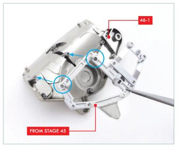
Position the left pelvic girdle **46-1** on your work surface and identify the fixing points for the pelvic frame (circled).
