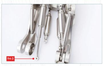
**STEP 10** Take the tendon **94-2** from this stage, with the **M3** nut. Fit the tendon assembly into the end of the muscle fitted in the previous steps.
