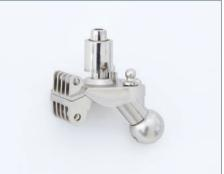
**STAGE COMPLETE!** The knee joint has been fitted to the lower end of the thigh. An ankle ball and socket have been fitted to the foot.
