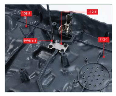
**STEP 3** Fix the connector **112-5** in place using four **PWB** 2 x 4mm screws.
