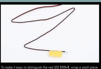
of masking tape around the cable, close to the connector.
