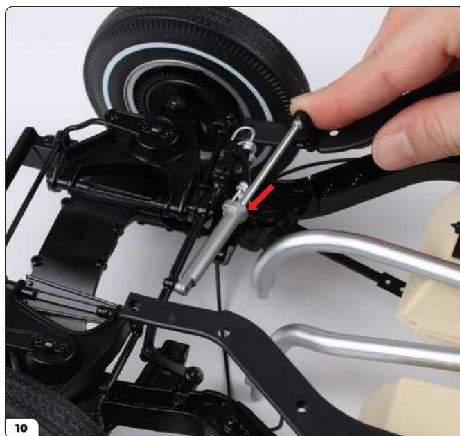
10 Push the cylinder bracket into the hole of the cylinder (arrow).
