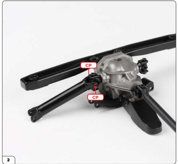
Secure using 2x CP screws.
