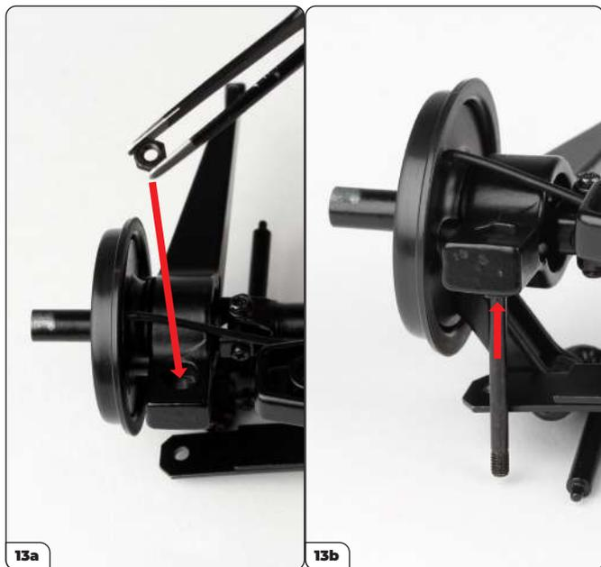
Flip the assembly over and place a hex nut into the left upper control arm (13a, arrow). Screw the long threaded end of the strut rod into the placed hex nut from underneath (13b, arrow) until the tip of the rod is flush with the nut.
