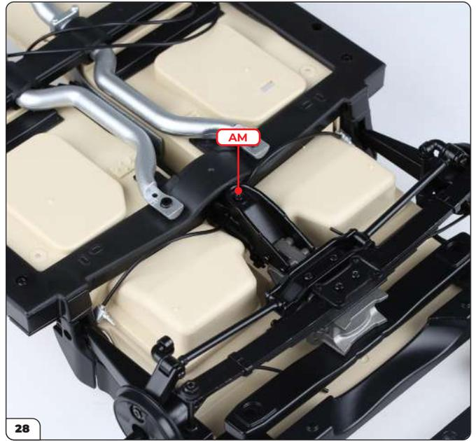
Start to secure the assembly by driving an AM screw through the support bracket.
