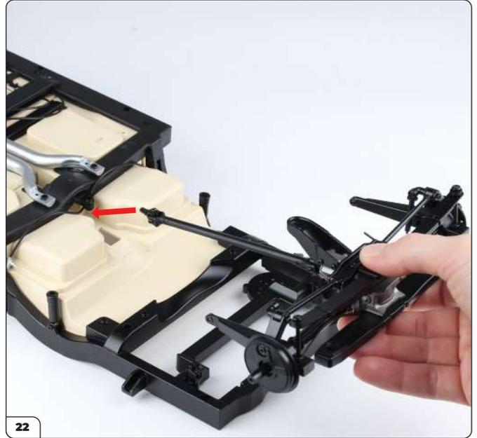
Align the rear suspension assembly with the rear chassis as shown. Fit the end of the transmission shaft into the central channel in the cockpit floor (arrow).
