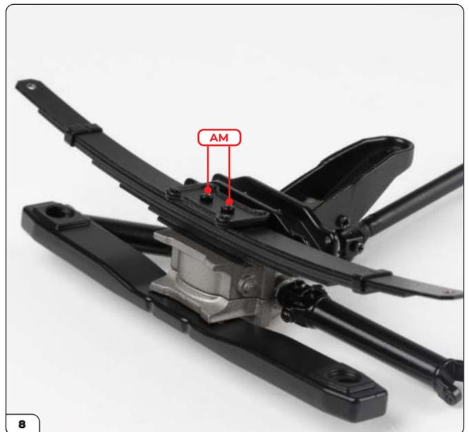
Secure using 2x AM screws.
