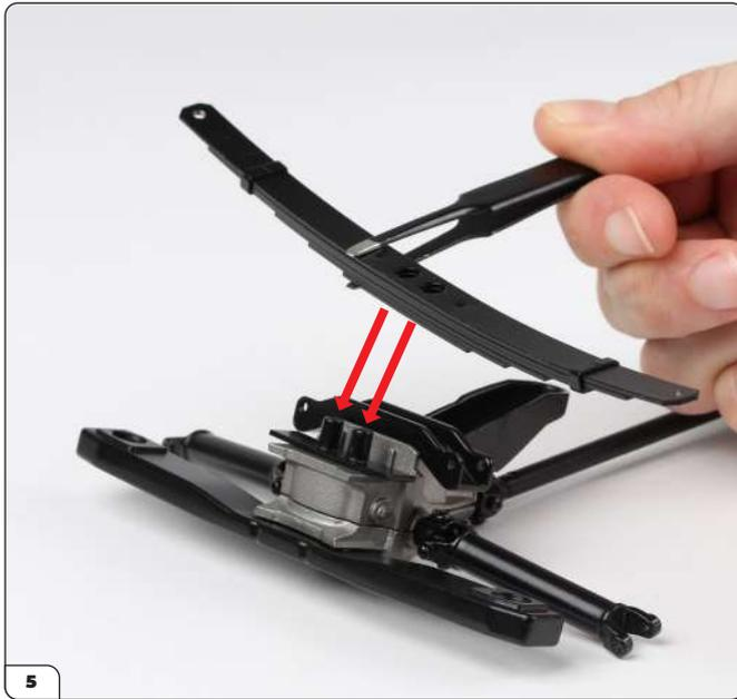
Fit the leaf spring in the orientation shown onto the fixing post (arrows).
