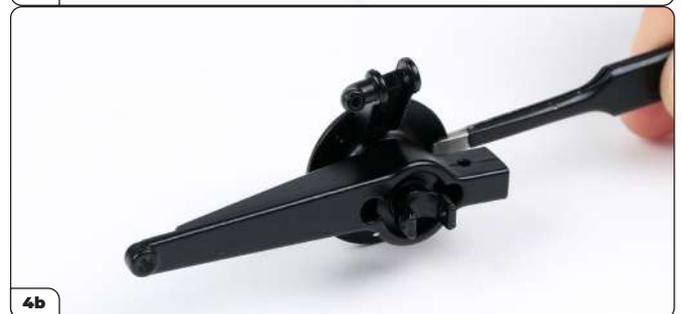
Align the left knuckle and upper control arm as shown (4a) then push screw posts of the knuckle into the holes of the arm (4b).
