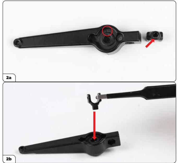
Take the left upper control arm (2a, marked with an 'L', circled) and a transmission shaft connector. Note it has a D-shaped post (2a, arrow). Fit the connector into the control arm (2b).
