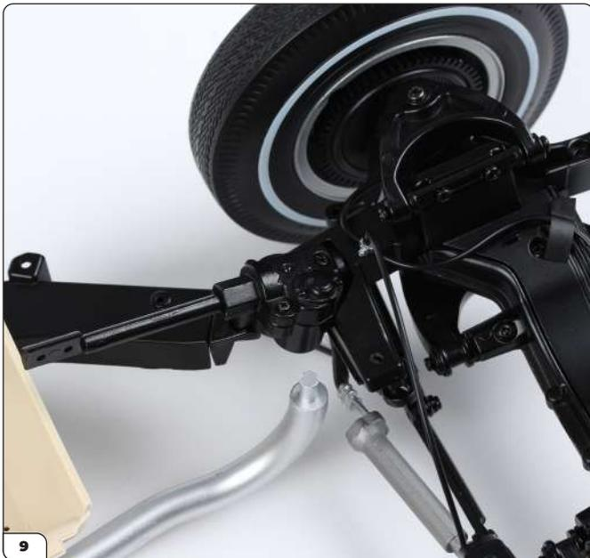
Place the gear box assembly into the recessed area as shown.
