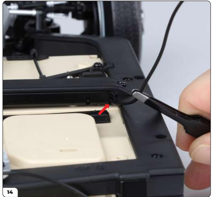
Plug the 145 mm long hose onto pin 1.
