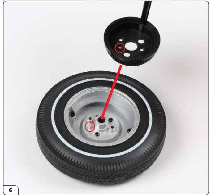
Fit the rear right brake drum onto the outer wheel rim using the locking pin and hole to align the parts correctly.
