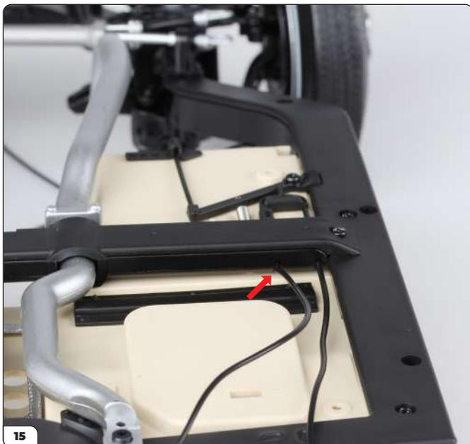
Plug the 285 mm long hose onto pin 2.
