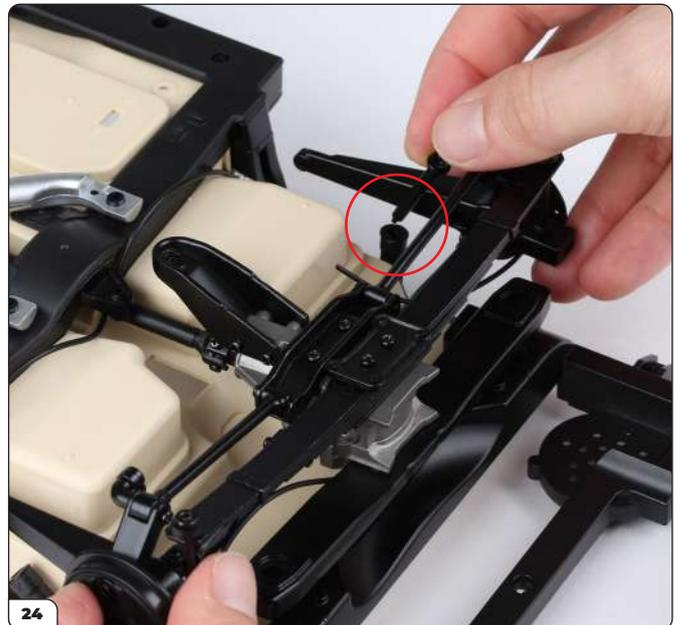
As you fit the assembly, guide the damper rods into the cylinders (circled).
