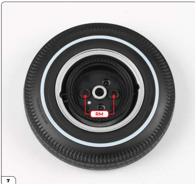
Secure using 2x RM screws.
