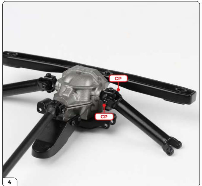
Secure using 2x CP screws.
