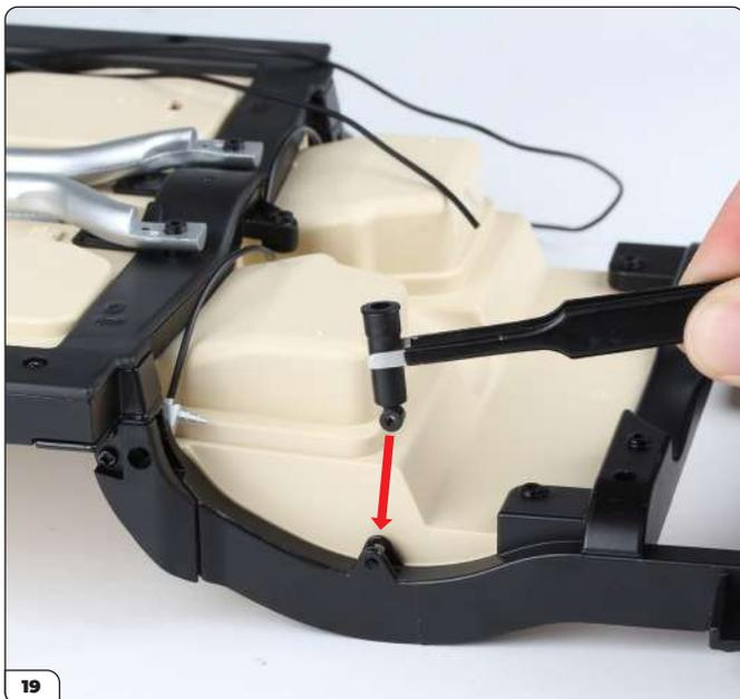
Fit a rear damper cylinder into the rear chassis as shown (arrow).
