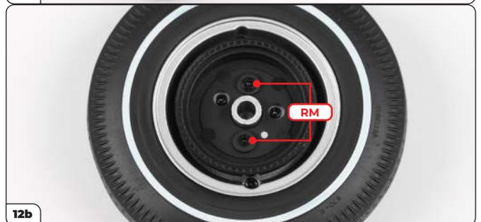
Retrieve the wheel assembled in stage 25. Fit the rear left brake drum onto the outer wheel rim (12a, arrow), using the locking pin and hole to align the parts correctly (12a, circled). Secure using 2x RM screws (12b).
