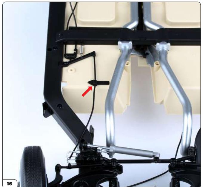
Plug the 76 mm long hose onto pin 3.
