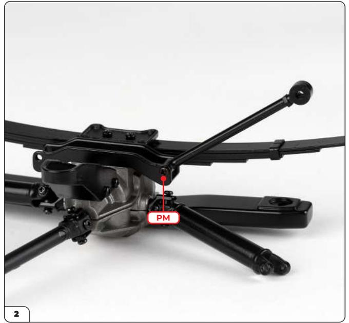
Secure using a PM screw.
