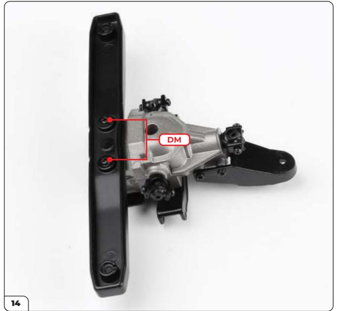
Secure using 2x DM screws.
