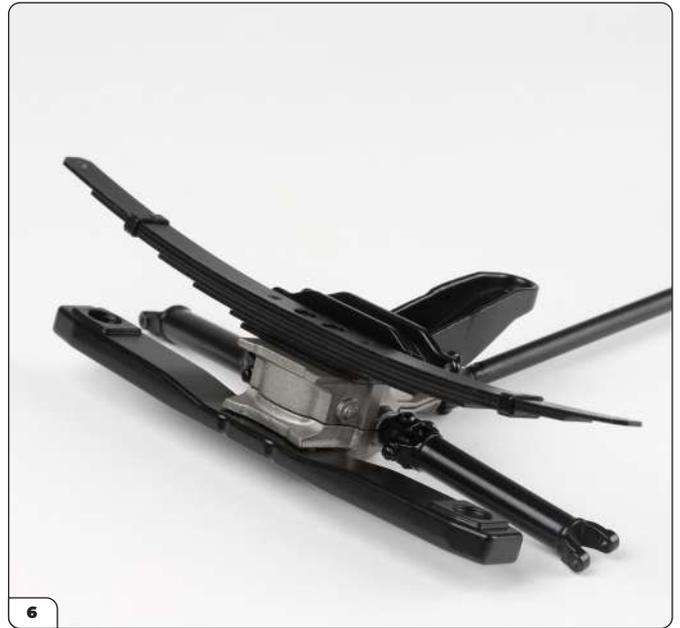
The leaf spring should curve upwards once in place.
