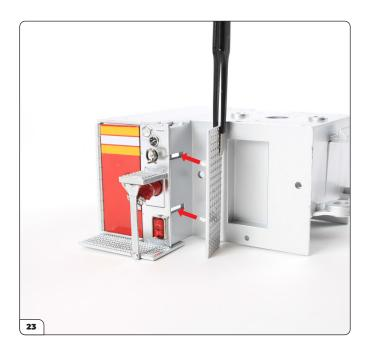
Take the left side panel and align the two tabs on the reverse side with the slots in the body midsection as shown. Note: the left side panel is wider than the right side panel - check you have the correct part.
