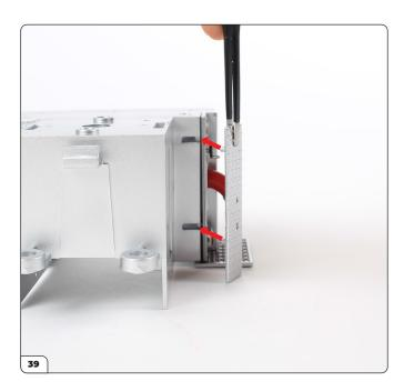
Line up the tabs on the reverse side of the right side panel with the slots in the midsection.
