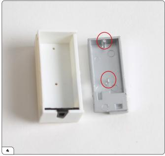
Take the electrical panel and note there are two pins on the reverse side (circled) that correspond with two holes in the electrical compartment.
