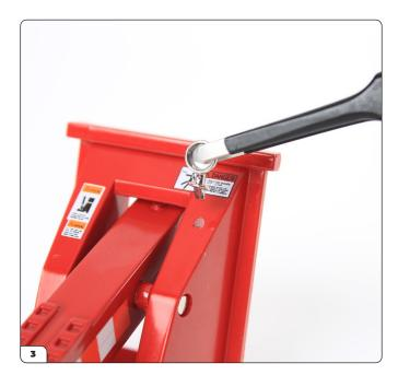
Line up the ground light with the D-shaped hole on the outrigger. The light should, of course, point down towards the ground. Apply a drop of glue to the peg of the ground light.
