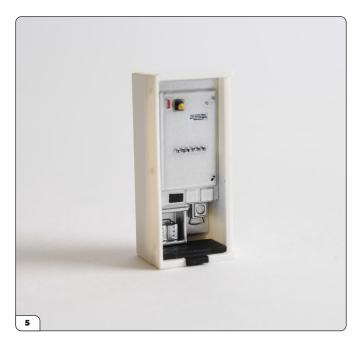
Press the electrical panel into place inside the electrical compartment until the pins on the reverse side are located firmly in the corresponding holes.
