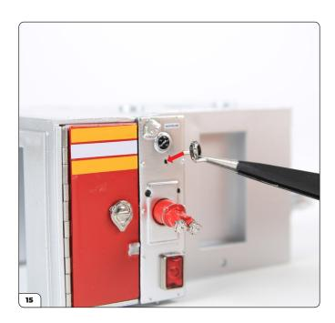
Take one of the supply valves and push it into the D-shaped hole on the water supply panel as shown. The fixing pin is placed centrally on the valve. Check you have it the correct way round.
