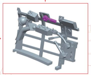
Glue the tailhook crank handle 024-02 to the right-side cockpit frame 022-01 assembled in stage 23.
