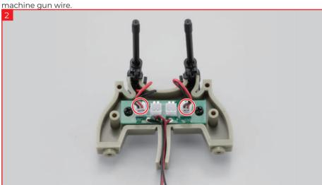
Push the machine gun wires into the outer sockets of circuit board 020-01. Note the orientation of the wires when plugging them in.
