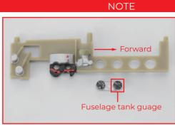
Place the instrument panel 024-04 in the direction shown and glue so that the guage with less scale on the dial (the fuselage tank guage) is on the right.
