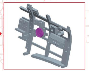
Glue the elevator correction wheel 024-03 to the left frame 024-01 of the cockpit.
