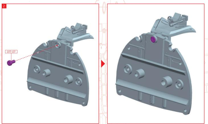
Fix the sighting device and machine gun cover in place using the screw 017-07 that came in stage 17.
