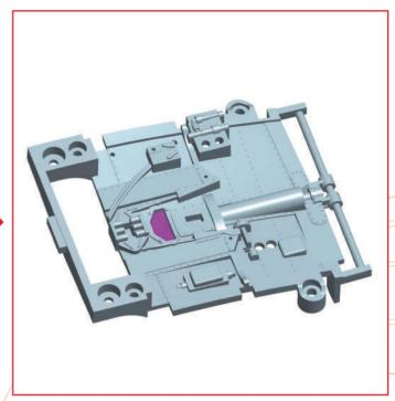
Glue window 018-02 from the underside of the cockpit flooring 018-01 with a very small amount of superglue. Be careful not to let the adhesive squeeze out.
