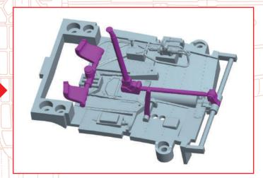
Glue the foot pedal 020-04 and the manual fuel pump handle 020-05 to the cockpit floor assembled in stage 18. The control stick and column 020-06 should be fitted but not glued.
