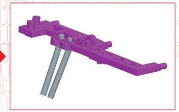
Glue the fuel tank switching pipe 025-05 to the instrument panel 024-04 assembled in stage 24. Be careful not to confuse the left and right as the thicknesses of the fixing pins is different.
