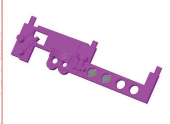
Push the hole of the fuel indicator 024-05 over the lug on the back of instrument panel 024-04 and glue in place.
