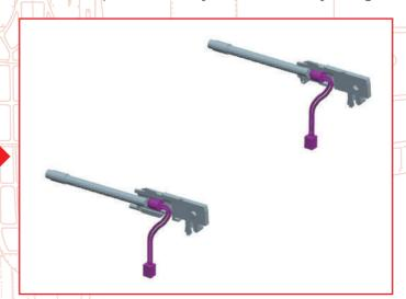
Insert LED **016-04** into each of the left and right units assembled in 1. Pass the wire through the notch at the bottom of the machine gun body.
