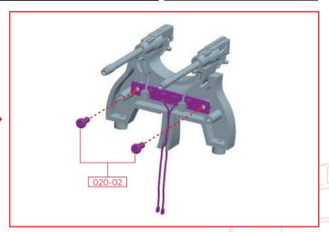
Fix the circuit board 020-01 to the machine gun assembly from stage 19 using two screws 020-02. Be careful not to pinch the
