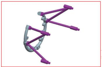
Insert the two pegs of the engine mount frame 017-01 and the engine mount frame 017-02 into the four holes of the engine mount ring 017-03. Glue together. Look closely at the image and pay attention to the top and bottom of the engine mount frame.
