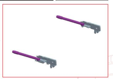
Fit the barrel **016-02** into the right machine gun body **016-01** and the left machine gun body **016-03**. Align the small peg on the barrel with the notch at the bottom of the machine gun body. The barrel does not glue.
