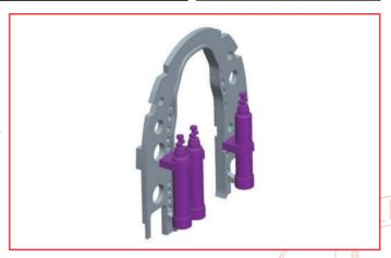
Glue oxygen tanks 026-01 & 026-05 onto the lugs at the bottom of the rear bulkhead 026-02. Check that tank 026-05, which is a 2-piece set, is on the left side of the cockpit.
