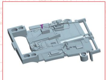
Glue the handle 018-05 to the cockpit floor 018-01 with a very small amont of superglue.
