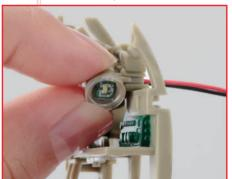
Thread the wire of the cockpit light 025-04 through the channel of the left-side frame 024-01 and push the light into place. It does not glue.
