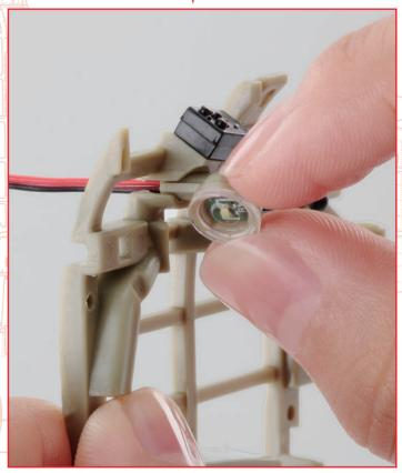
Thread the wire of the cockpit light 023-04 through the channel in the hole of frame 022-01 and push the light into place. It does not glue.
