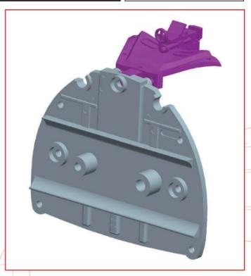
Fit the sighting device and machine gun cover assembled in stage 17 to the front bulkhead 019-01.
