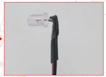
Bend the LED 016-04 to form a right angle. Hold the base of the LED with needle-nose pliers and carefully bend the wire with your fingers.
