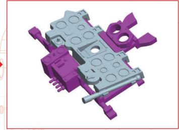
Glue the instrument panel assembled in 1 to the frame 021-02. Pay attention to the orientation and the areas to glue. The instrument panel and 021-02 are glued at a slight diagonal.
