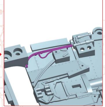
Glue piping 018-03 to the cockpit flooring 018-01 with a very small amount of superglue. Be careful not to let the adhesive squeeze out.
