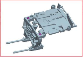
Secure the machine gun and cockpit floor with the two screws 018-06 that came with stage 18. Be careful not to trap the wires on the board.
