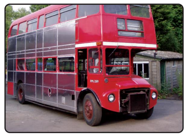
A photograph of RML2589 during restoration, showing the radiator in position at the front of the bonnet.
