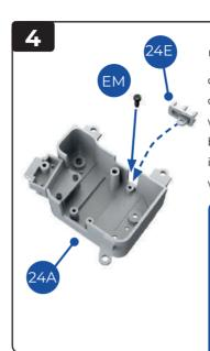
Looking at the inside of the gearbox casing 24A, position the tab on the cover 24E through the slot in the casing, over the screw hole. Fix the cover in place with an EM screw. Turn the casing over (see below) and fit the pegs on the valves 24D into the sockets in part 24A. Fix in place with two AP screws.
