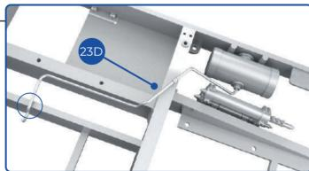
Take the line 23D and check the shapes of the ends and the position of the pin in the centre section, to ensure you get it the right way round. Fit one end of the line into the socket on the tank 23B, and fit the pin into the hole in part 17A. The inset above shows the line in place – the free end of the line fits over a strut in the frame (circled). Use a small piece of masking tape to hold the line in place temporarily.
