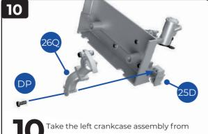
Take the left crankcase assembly from the previous stage and identify the fixing point for the oil filler neck 26Q on the injection pump 25D. Fix in place with a DP screw.
