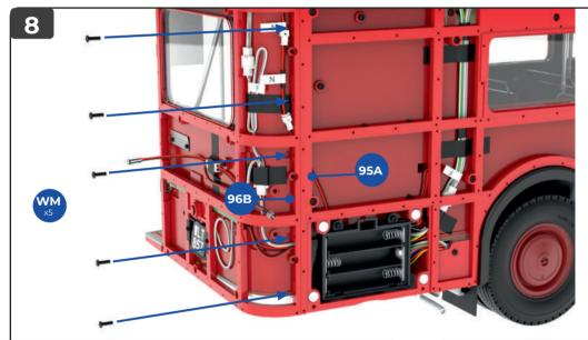
At the rear right corner, fix the side of the rear frame
