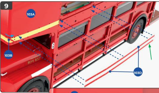
The two side strips **103D** are fitted next. Fix them one at a time. Note that there is a wider gap between the screwholes towards the rear of the model (green arrow).
