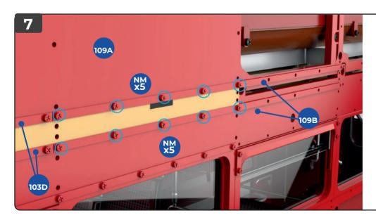
Fix the left-hand ends of the two side strips **109B** in place, ensuring that they continue the line from strips **103D**. You will need five red **NM** screws for each strip.
