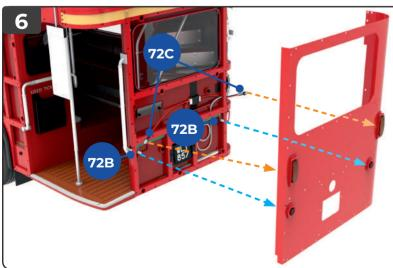
Position the rear wall panel **107A** against the back of the model. As you do so, fit the lamps into the sockets on the rear panel (circled below) as follows:
