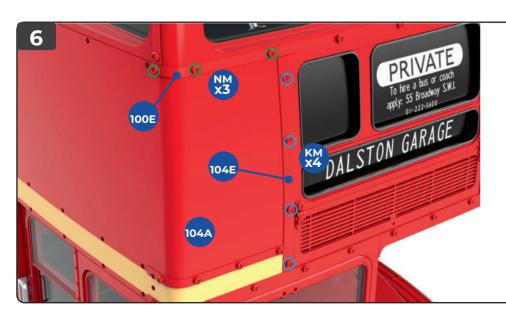
Fit the strip **104E** in place using the four **KM** screws removed in step 1 (circled in light blue). At the top of the corner panel **104A** fix the front strip **100E** in place, with three **NM** screws (circled in green), wrapping the end around the corner.
