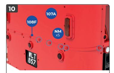
Continue fixing the trim **108F** in place on the right-hand side of the rear wall panel **107A**, wrapping it round the curve of part **107A**. You will need to use five more red **NM** screws. Note that there are two screw holes quite close together between the indicator and brake lights.
