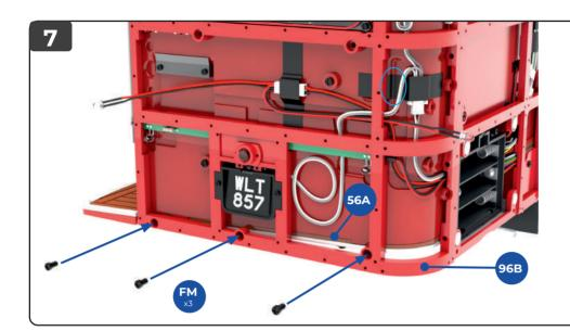
The rear framework is fixed in place with **FM** and **WM** screws. Starting at the lower edge, fix the frame **96B** to the rear platform **56A** with three **FM** screws. Note that there is still a recess for the indicator housing (circled in light blue).
