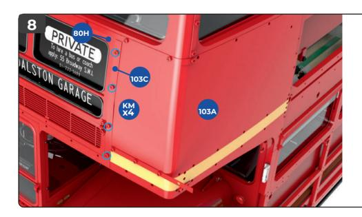
Position strip **103C** down the side of the destination blind, just overlapping the edge of the front corner panel **103A**. The strip is not symmetical, so ensure that you have it the right way round. Fix the strip to the front blind frame **80H** with four red **KM** screws (circled).
