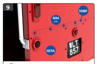
Position the first strip **108F** (marked A177) across the rear of the model above the brake lights, with screw holes aligned. Note the more even spacing of the screw holes at the left-hand end of part **108F** (see also next step). Use four red **NM** screws to fix the left-hand end of the trim in place.
