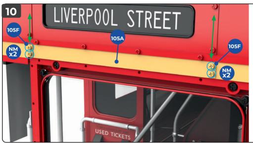
The two cream strips 105F (marked A167B) are positioned vertically across the cream band at the rear of the bus, on either side of the destination blind area, so that they continue the line of the vertical strips fitted in steps 5 and 6 (green arrows). Fix each of them in place with
