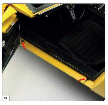
Place the assembly upright on your work surface and open the driver's side door. The T-shaped protrusions fit into shaped recesses in the door sill (arrows).
