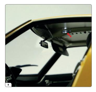
While either or both of the doors are open, the interior light on the roof will illuminate.
