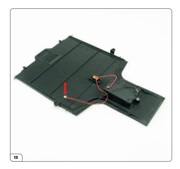
Next retrieve the bottom floor panel. The switch has a loose plug (arrow) to connect to the circuit board before fitting the panel.
