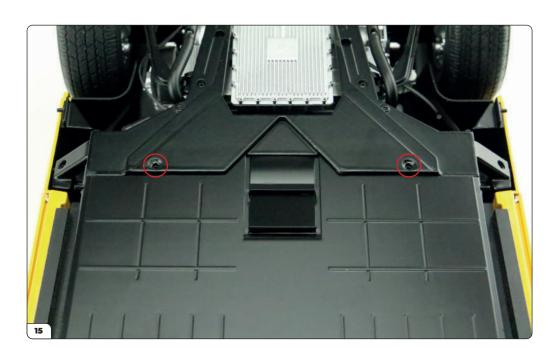
Position the bottom floor panel by fitting the wider end into place towards the rear end of the model; this fits just under the rear frame near the engine. The two screw holes in the floor panel must be aligned with the holes in the rear frame (circles).
