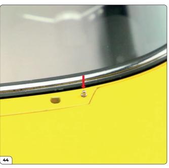
Fit the remaining washer nozzle into the left-hand side hole in the same way.
