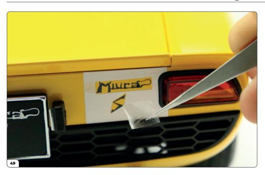
Press firmly down on the two stickers to ensure they have adhered, then slowly remove the transparent film that protects the stickers using a pair of tweezers. You may wish to have a cocktail stick to hand in order to gently press the sticker back if any part of it begins to peel away with the film.
