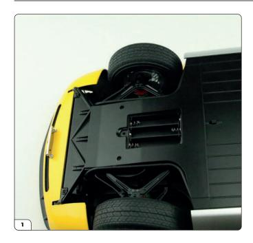
To insert the batteries, turn the model over and remove the battery compartment cover. To do this, you have to loosen the cover screw with a Phillips screwdriver.
