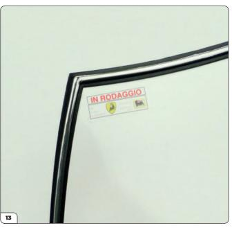
Place the sticker as shown in the windscreen's upper corner on the passenger side. Make sure the area is clean of any dust or fingerprints before sticking.
