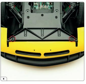
Carefully turn the assembly over then fit the two mounting brackets onto the screw holes in the frame (circled).
