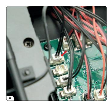
Plug the left headlight into connector 9 (arrow).
