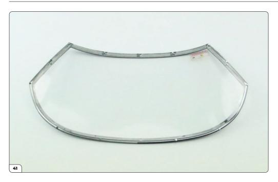
Once the tape is in place, peel the paper off each piece to reveal the adhesive as shown.
