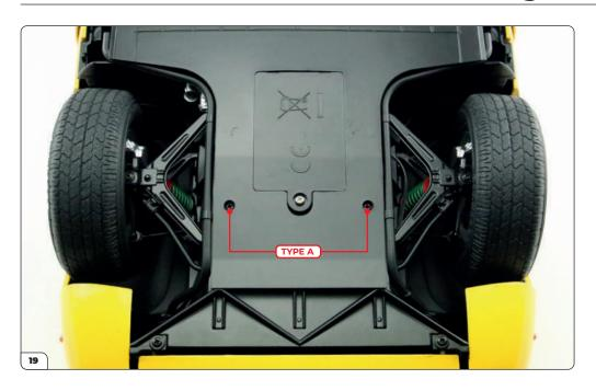
Finish fixing the floor panel using 2x Type A screws (supplied with Stage 97) in the holes located either side of the battery compartment.
