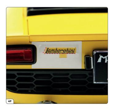
Take the logo transfer sheet (supplied with Stage 1) and use a pair of scissors to separate the 'Lamborghini' sticker from the 'Miura S' sticker. Carefully peel the 'Lamborghini' sticker from the sheet and apply it to the left side using the template as shown. Use the angled edge on the left to align the 'L', then the horizontal edge to the guide the underline as indicated by the dashed lines.
