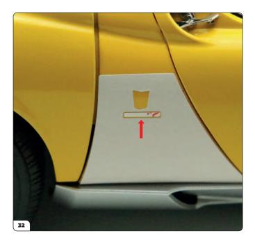
Using the template as a guide, position the tape onto the body (arrow). Once in place, remove the paper from the adhesive.
