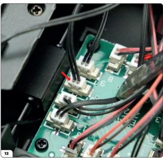
Repeat steps 9 and 10 for the left head light then plug it into connector 10 (arrow).
