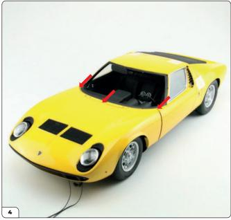
Fit the front body onto the main assembly and position it so it aligns with the central body (arrows).
