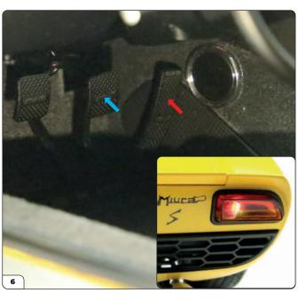
Pressing the accelerator pedal (red arrow) will activate the acceleration sound. By pressing on the brake pedal (blue arrow), the taillights will illuminate (inset).
