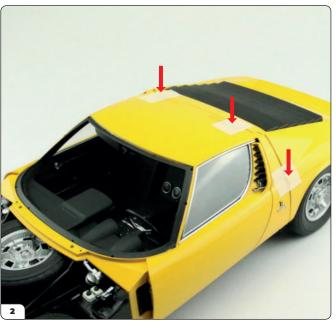
Place the main assembly nearby on your work surface and ensure the rear body is secured by masking tape (arrows).
