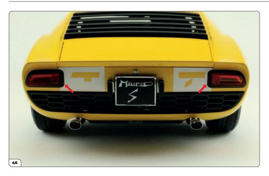
The last few steps are to apply the logos to the rear of the model. First, take the rear logo templates and separate them from their backing. Apply them to the rear body as shown, using the taillights as a guide for fitting them in place (arrows).
