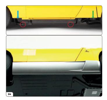
Take the left side skirt and secure it in place under the driver's side door. Start by aligning the two holes on the lower edge of the skirt with the pins (circled, top image) and then pushing all the joints into their positions at the same time.
