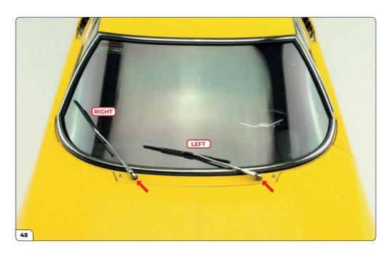
In the larger shaped holes located next to the washer nozzles, fit the windscreen wipers (arrows). The wipers are supplied in bags marked 'R' and 'L' to distinguish the right from the left.
