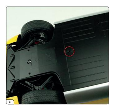
Replace the battery compartment cover and tighten the screw. Flip the switch from 'OFF' to 'ON' (circled).
