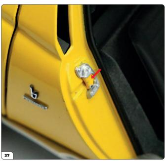
Next you'll install the shims to the door. Open the right side door and locate the space indicated by the arrow.
