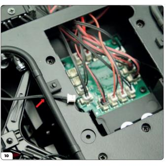
Carefully lift up the radiator pipe and fit the plug through it (arrow). Pull the wire through then press the radiator pipe back into place.
