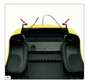
Turn the front body over, then lift up its two mounting brackets (arrows). Make sure to move the headlight wires towards the front and out of the way as shown.
