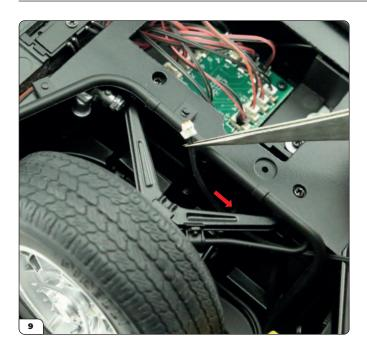
To connect the headlights, first locate the plug from the left headlight and pass it under the suspension arm (arrow)..
