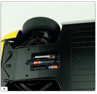
Insert three AAA batteries, orienting them as indicated by the markings inside the battery compartment.
