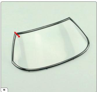
Turn the trim over so the front is facing you as shown. You'll now apply the "In rodaggio" sticker to the windscreen, which is positioned on the passenger side (arrow).
