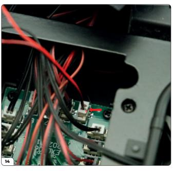
Guide the wire under the crossbar as before and plug the switch into connector 5 (arrow).
