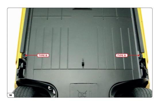
Drive 2x Type B screws (supplied with Stage 97) into the raised screw holes either side of the floor panel.
