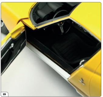
The left side skirt should look like this once fitted. Fit the right side skirt in the same way on the passenger's side. If either of them are difficult to fit in place, check the fixing points for excess paint and remove if necessary.
