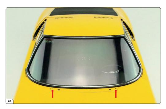
Press the pins highlighted in step 40 into the holes highlighted in step 39 to fit the windscreen. Push down firmly on the sections with double-sided tape to adhere the windscreen in place. Note the two small holes indicated by the arrows for the next step.
