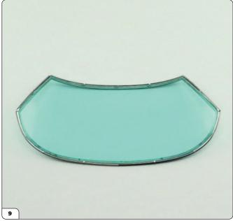
Now take the windshield, which is covered with protective films: one transparent and one green. Remove the transparent protective sheet. Be sure to handle the windscreen by holding it by the outer edges to avoid leaving fingerprints on the unprotected surface.
