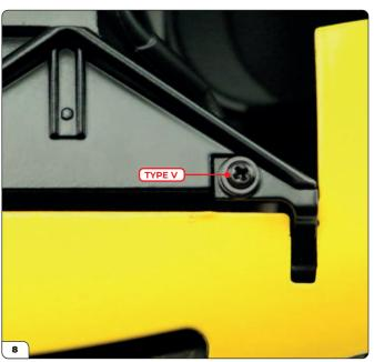
Use a second Type V screw to secure the right mounting bracket.
