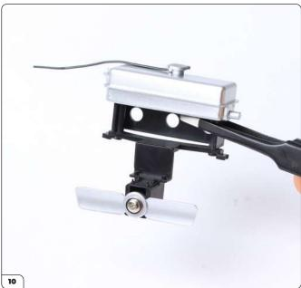
Press the parts firmly together and secure them in place using 2 x AG04 screws.
