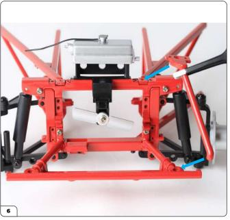
Take the front subframe left stay and align it with the subframe as shown. The three holes at the wider end fit next to the header tank support; the opposite end angles downwards and fits into the hole on the front subframe base.
