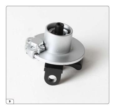
The brake disc and caliper are correctly positioned on the suspension upright. Check that the underside of the caliper fits onto the locating pin.
