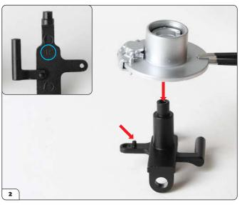
Fit the brake disc onto the central part of the right suspension upright, ensuring that the caliper is aligned with the locating pin.
