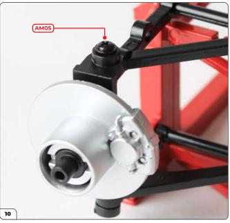
Secure the suspension bush in place with another AM05 screw. Again, do not overtighten the screw as the upright must be free to turn.
