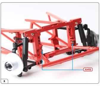
Fit the screw mounts on the subframe base into the corresponding recesses on the assembly and secure in place using 2 x AM15 screws.
