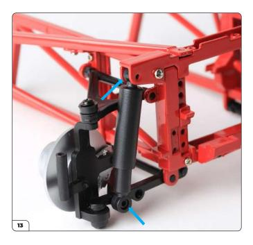
Take the shock absorber assembly and fit one end to the subframe, and the other end to the lower wishbone as shown.
