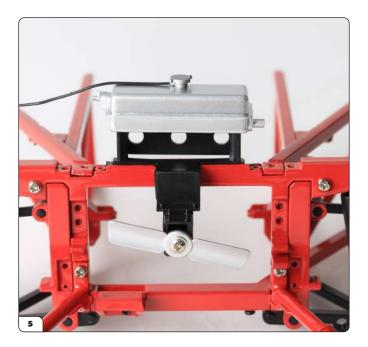
Press the header tank firmly into place.
