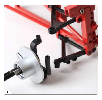
Align the brake disc assembly with the upper and lower wishbones on the subframe.
