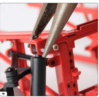
Squeeze the pin with pliers to press it fully into the hole.
