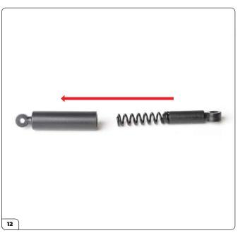
Take the shock absorber shroud, coil spring and damper body and arrange them as shown. The damper body fits into one end of the coil spring and the other end of the spring fits into the shock absorber shroud.
