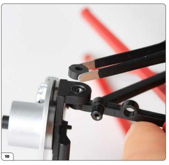
Fit the other suspension bush over the hole and the tip of the lower wishbone.
