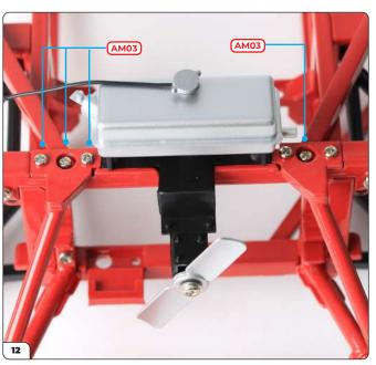
Use 3 x AM03 screws to fix the right stay to the top of the subframe. Finally, screw another AM03 screw into the left stay so that 3 x AM03 screws now secure the left stay in place on the subframe.
