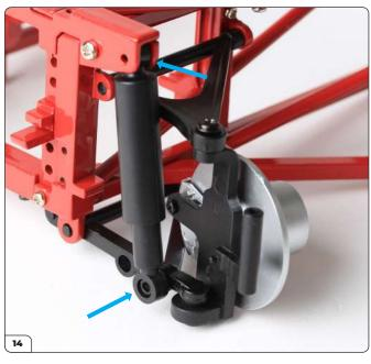
Take the shock absorber assembly and fit one end to the subframe, and the other end to the lower wishbone as shown.
