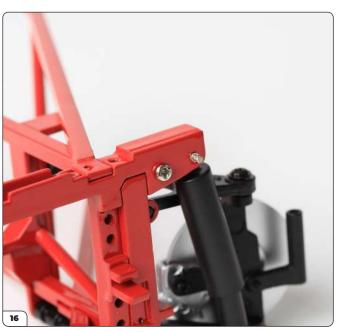
Push the pin in to secure the shock absorber in place.
