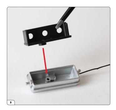
Fit the header tank support to the header tank, aligning the raised screw sockets.
