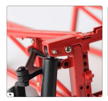
Push the pin in to secure the shock absorber in place.
